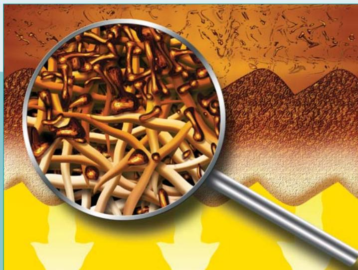
**Adsorption of oil degradation products (Varnish)**
