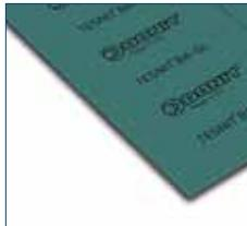
TESNIT® BA-GL combines excellent thermal and chemical resistance with outstanding mechanical properties, especially bolt torque retention. Thus, TESNIT® BA-GL is particularly suited for gas and steam supplies, heating systems, pumps and compressors.
