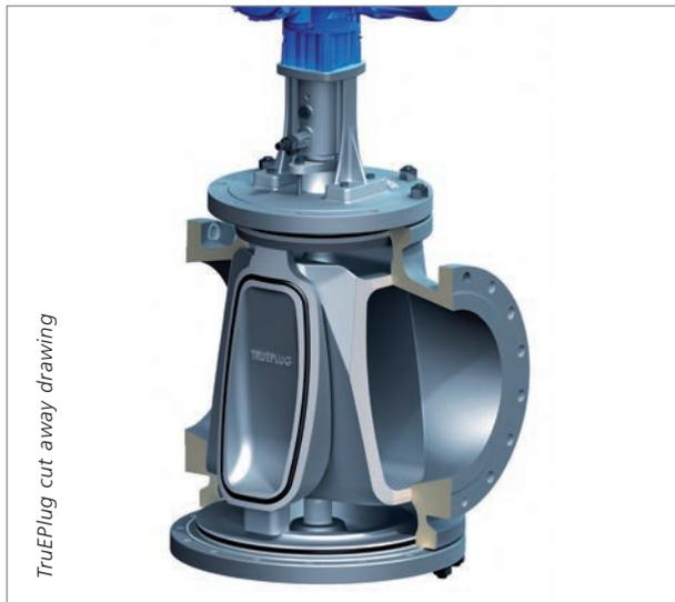
As the plug lifts and rotates from the open to the closed position, clearance is maintained between the plug shield and the valve body, allowing free movement and avoiding scoring.
