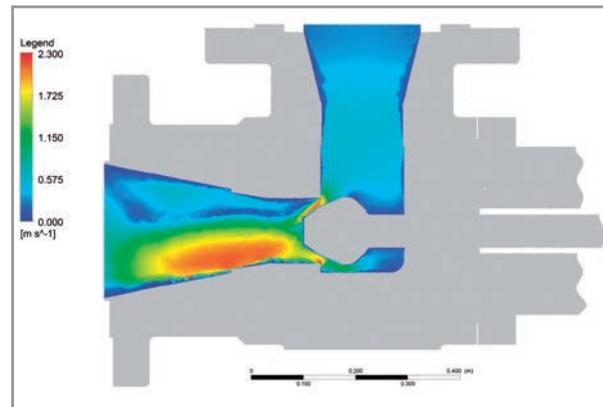
Simulation is at the heart of control valve design for difficult applications. Many negative process consequences such as flashing, crystal formation, or sediment deposits are either avoided or accommodated in SchuF control valve design through extensive use of FEA and CFD (ANSYS) simulation.
