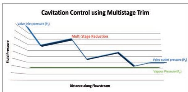
This is achieved by using a multiple stage trim that reduces the pressure drop in stages. The principle is illustrated in the above diagram, where pressure is let down in three successive stages. SchuF has a broad range of multistage trims that allow pressure to be let down in up to six stages in a step plug, or more in a stacked cage design.
