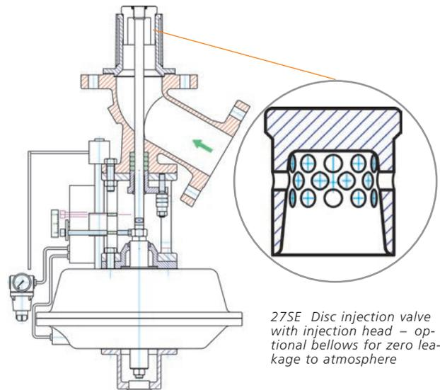
27SE Disc injection valve with injection head – optional bellows for zero leakage to atmosphere
