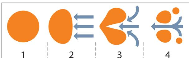
Micro jets have a velocity of 400 km per hour and temperatures of up to 5,500 °C and literally blast away pieces of the valves components or lead to severe pitting and accelerated corrosion. Cavitation is typically accompanied by accentuated hydrodynamic noise and vibrations in the valve and piping.
