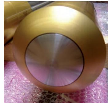
Piston head with tungsten carbide coating
