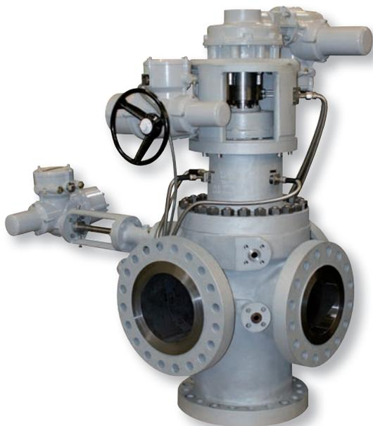
The SwitchPlug consists of only a few moving parts – body, plug and actuator – and is therefore highly reliable. There is no gap between the plug and the valve body where the fluid or coke particles can settle, damage piping or score the valve. Flushing is therefore only required while the plug is in motion.
